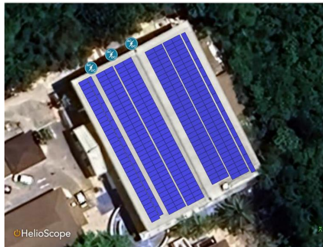
Figure 4: Solar Panels Placement
