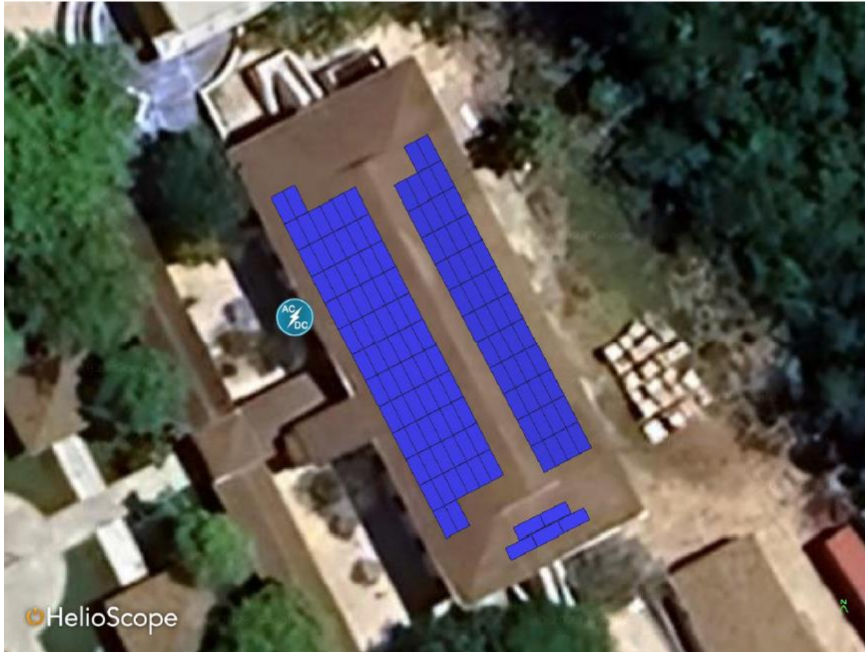
Figure 5 Solar Panel Placement of Admin Block
