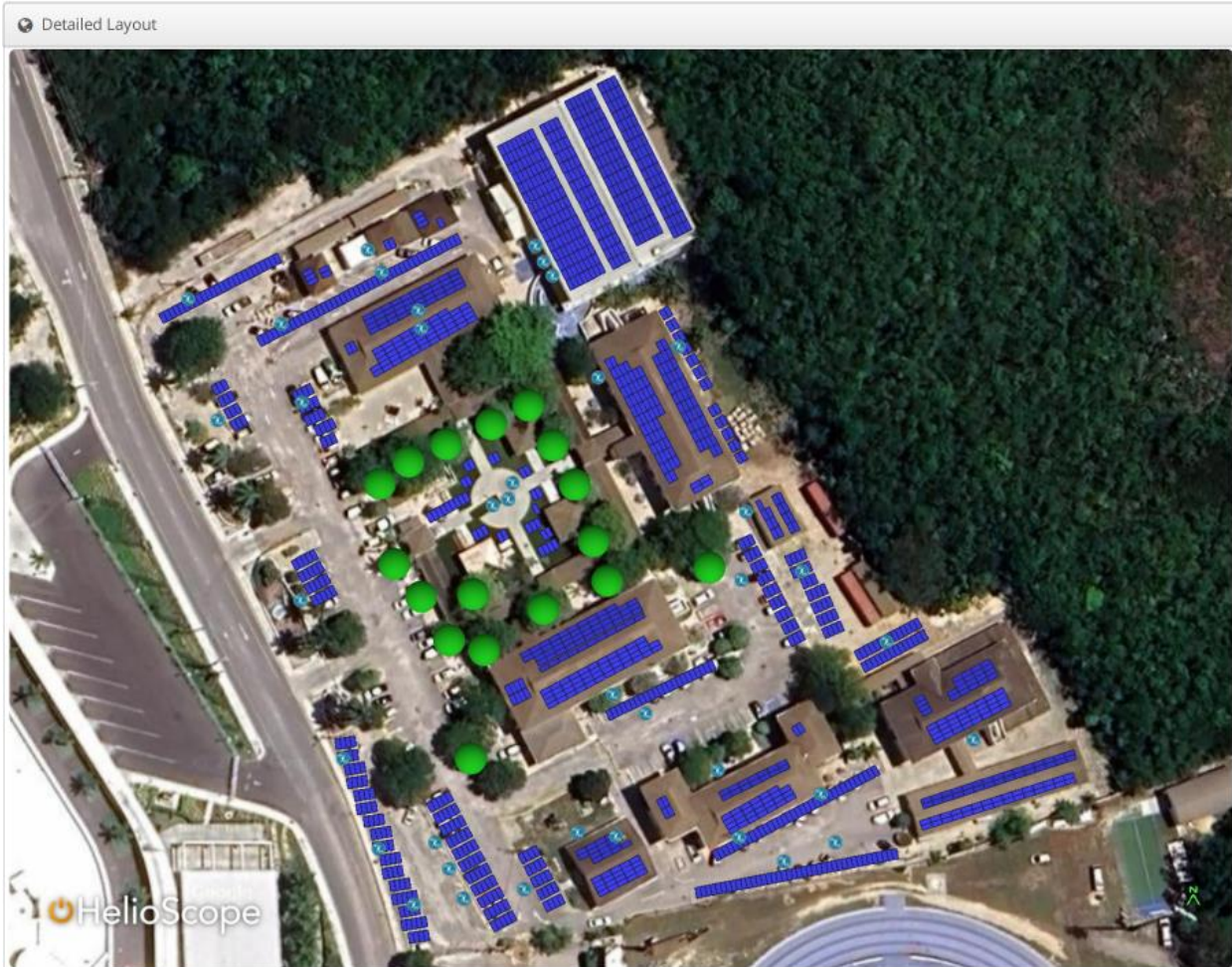
Figure 1: Solar Panels Placement
